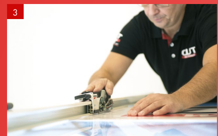
3 Pull the cutting head towards you.
