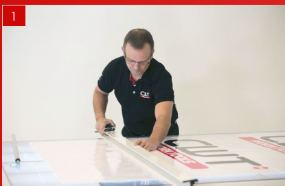
1 Place the Linear cutter into position.
